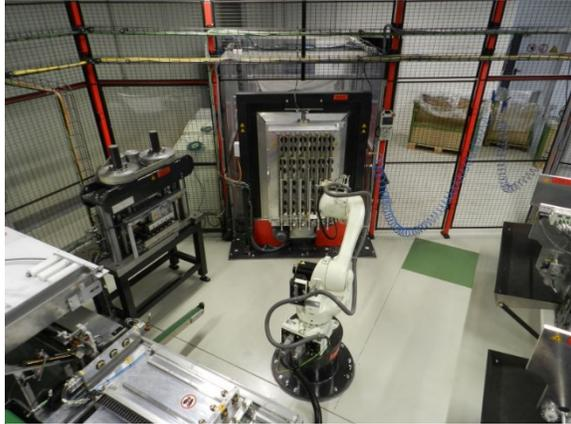
*The central RS020N robot supplies the prepared pipes to a specifically designed Kawasaki milling robot.*
