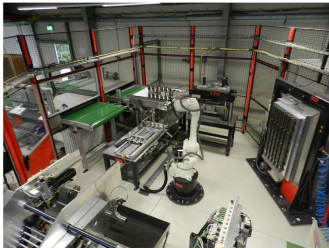
*The Kawasaki robot RS020N verbindet connects all steps of the process within the cell.*
