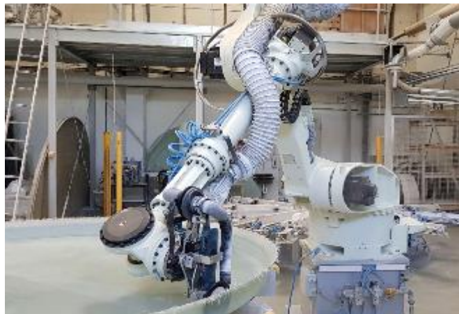
The Kawasaki ZT130L working the edge of a tank bottom.
