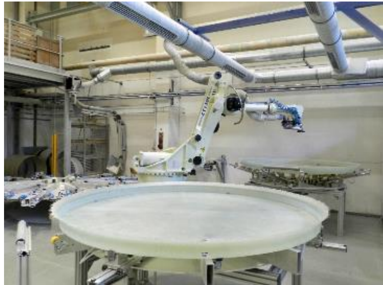
The system based on the Kawasaki robot allows fast and flexible processing of the tank lids and bottoms in series production.
