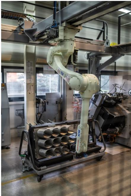
*The Kawasaki RS010L precisely feeds the finished bent parts into a register.*
