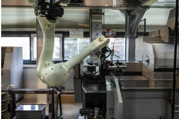
*The robotic cell can be adapted to new productions in the shortest possible time thanks to a quick gripper change and the possibility of attaching different parts.*
